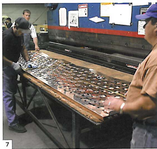
6: An extensive series of mock-ups were created by A.Zahner for design review by Herzog and de Meuron. This image shows a mock-up of panels for the overhang being reviewed for the resultant shadow patterns cast by multiple layers of perforated copper.
